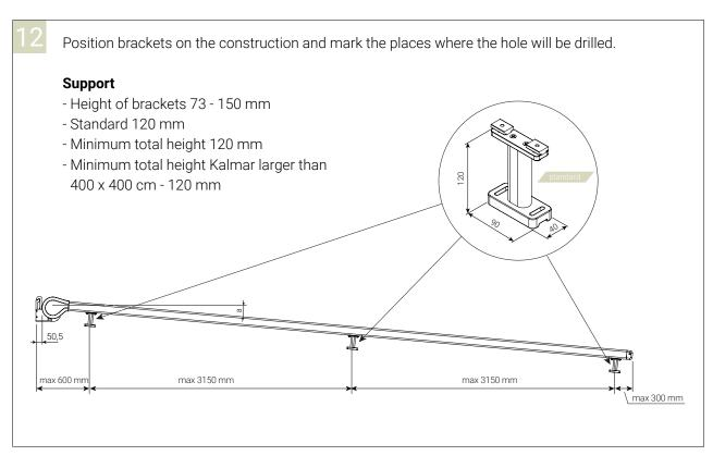
Regulation must be done very carefully. Difference between dimensions cannot exceed 5 mm! It is important to check the dimension between guide rails by the box and at the plugs of the side guide rail - dimensions have to be identical. Not following the rules during installation may cause damage to the product and invalidate the warranty. This may even cause accidents!
