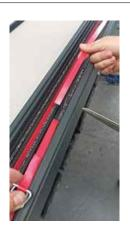
After correct installation, perform a test run, check the fabric tension, check the lines in the guide rail for tension and correct operation (if they did not fall off the guide wheels).
