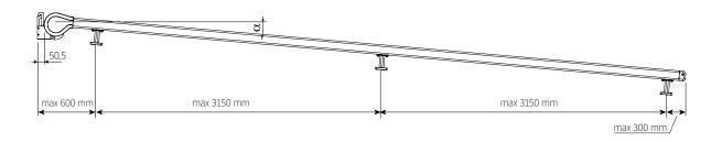
**CAUTION!** Risk of the awning falling, the order of assembly must be observed! Evaluate the conditions on location and use the appropriate fixings. Don't do the work by yourself, remember to use a level during installation.
